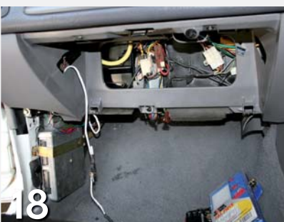
▲ Once out, we fed the wires and control switches under the dash and through the sides
