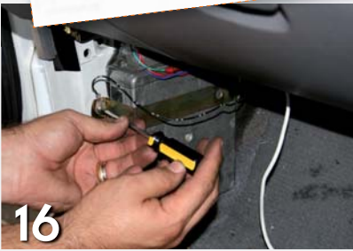
▲ Put the ECU back in its original position making sure to mount the earth connection
