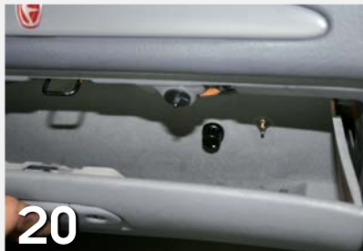
▲ We decided to mount the switch and potentiometer in the glovebox for a couple of reasons. 1. It's neatly hidden. 2. Will stop the kids or mates from playing with the settings!
