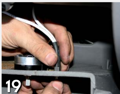
▲ We then drilled two holes for the control switches and mounted them
