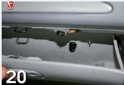
▲ We decided to mount the switch and potentiometer in the glovebox for a couple of reasons. 1. It's neatly hidden. 2. Will stop the kids or mates from playing with the settings!
