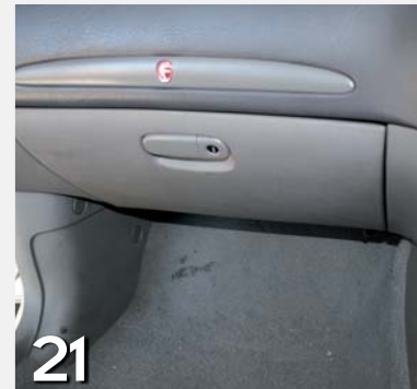
▲ We then refitted the kick panel, glovebox and scuff plate for a stealth installation
