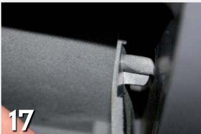
▲ Remove the glovebox by releasing the two side tabs
